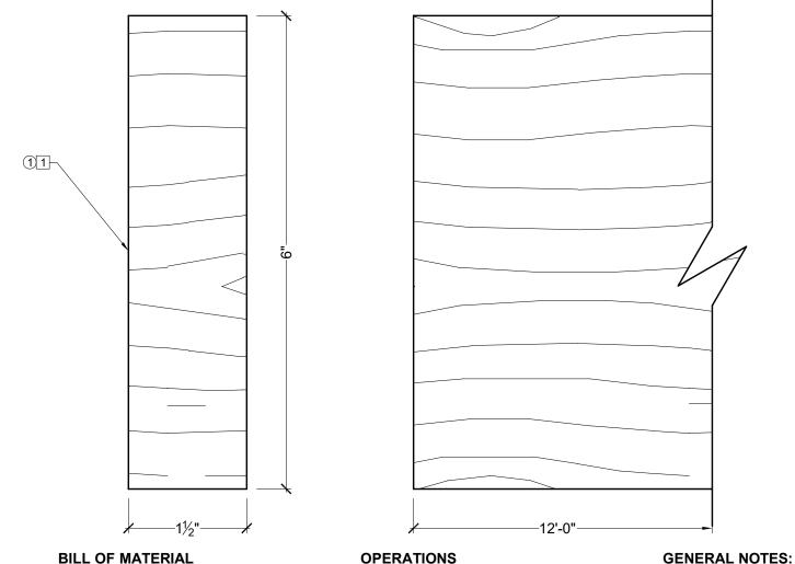
1 MD1108-6RS - MOULDING MADE OF POLYURETHANE.
